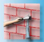
AQUIA-PLUG, leak stopping cement, is a fast setting hydraulic compound used for filling holes, cracks or leaks in masonary floors and walls. AQUIA-PLUG sets under water and is the ideal cement for stopping water infiltration.
